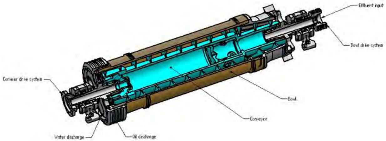
Fig. 1 General configuration of a centrifugal separator
